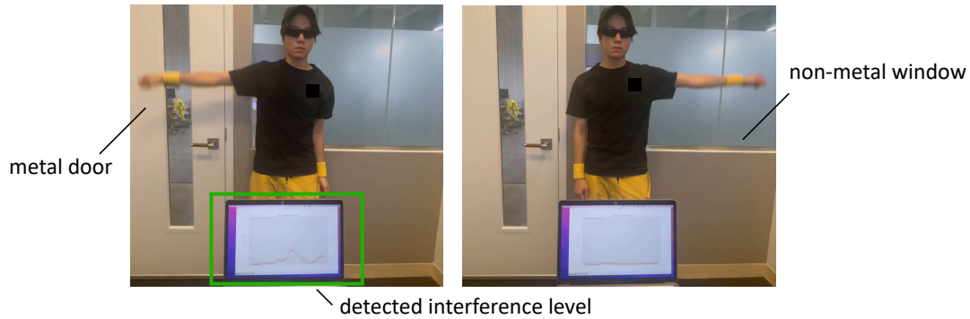
Fig. 11. Demonstration of the interference detection. The interference level is estimated on a frame-by-frame basis and displayed on the laptop (red line). When the sensor passes near the metal object (left figure), the interference level increases, while it remains unchanged in other situations (right figure).
