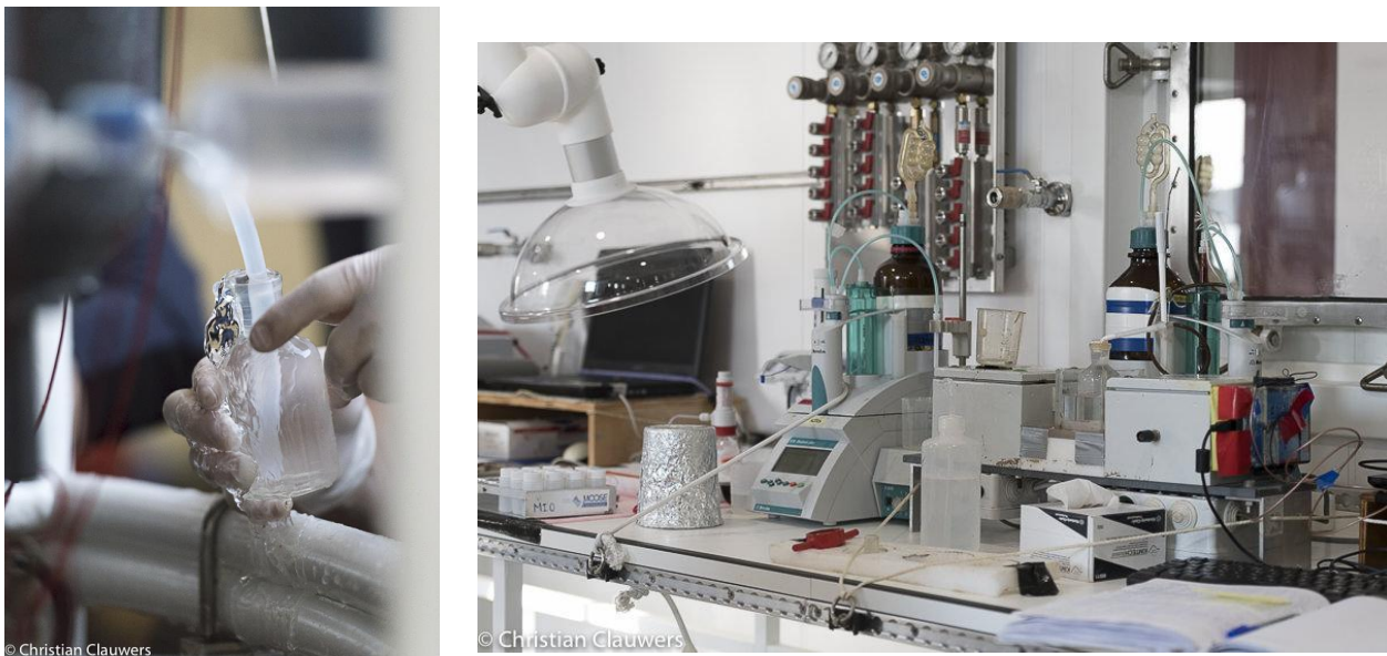
Figure 16. Sampling detail and Winkler titration system used during the cruise. Credit: C. Clauwers.
