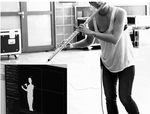
Figure 3: Tracking a moving instrumentalist. Inset a view of the camera analysis tool. Note the failure of the kinect to capture the shiny surface of the flute.
