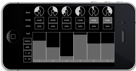
Figure 1: A mixer interface in Control with volume, pan, mute and solo controls for six channels.
