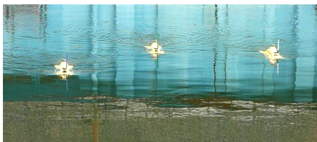
Fig.8 Centralized formation control of three AUV's
