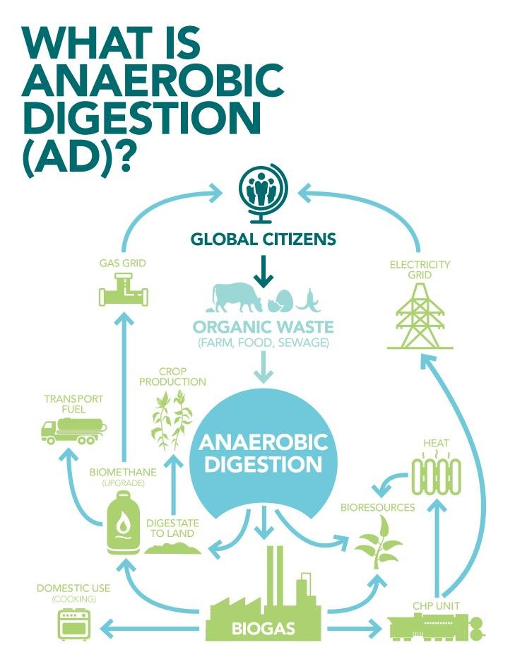
AD is a natural process in which microbes digest plant material in sealed containers, producing biogas which can be used for cooking, heating, cooling and electricity production or upgraded and used for vehicle fuel or gas grid injection. Biogas is a mixture of methane, carbon dioxide and other gases. A co-product of the anaerobic digestion process is a biofertiliser called 'digestate', containing water, crop nutrients and organic carbon for
