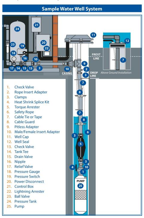
This illustration is intended to represent some of the components that can be included in a water well system and is not intended as an installation guide.
