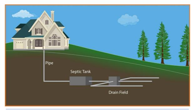
This image is intended to represent some of the components that can be included in a septic system and is not intended as an installation guide. Check local codes for actual requirements and restrictions.
