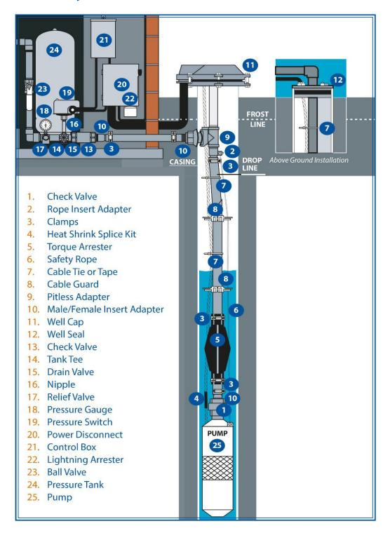
This illustration is intended to represent some of the components that can be included in a water well system and is not intended as an installation guide.
