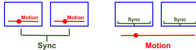
Fig. 3 Blue rectangles represent media components, red symbols represent motion, and green symbols represent the process of media synchronization. To the left: internal timing and external media synchronization. To the right: external timing and internal media synchronization.
