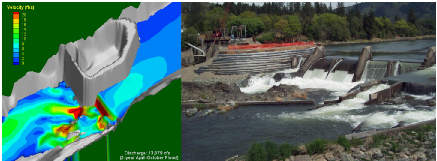
Figure 2.—Left: SRH-2D predicted flow velocity at the Savage Rapids Dam during the right cofferdam construction and a 2-year flow event (~14,000 cfs). Right: View of actual field conditions in May 2009 (5,100 cfs). A flood occurred a few days later at 11,200 cfs and the cofferdam failed exactly where the 2D model predicted high velocity. This resulted in the contractor using the model output to guide design improvements.
