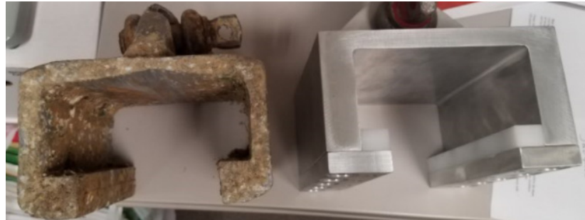
The log boom anchors are cut from a large block of material, resulting in material waste and manual labor. After approximately one year in service, the log boom anchors become worn and corroded and need to be replaced.
