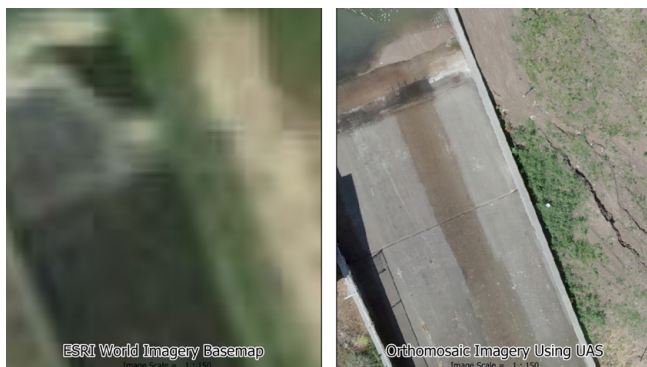
A comparison of available imagery between ESRI World Imagery Basemap and orthomosaic imagery captured by UAS.
