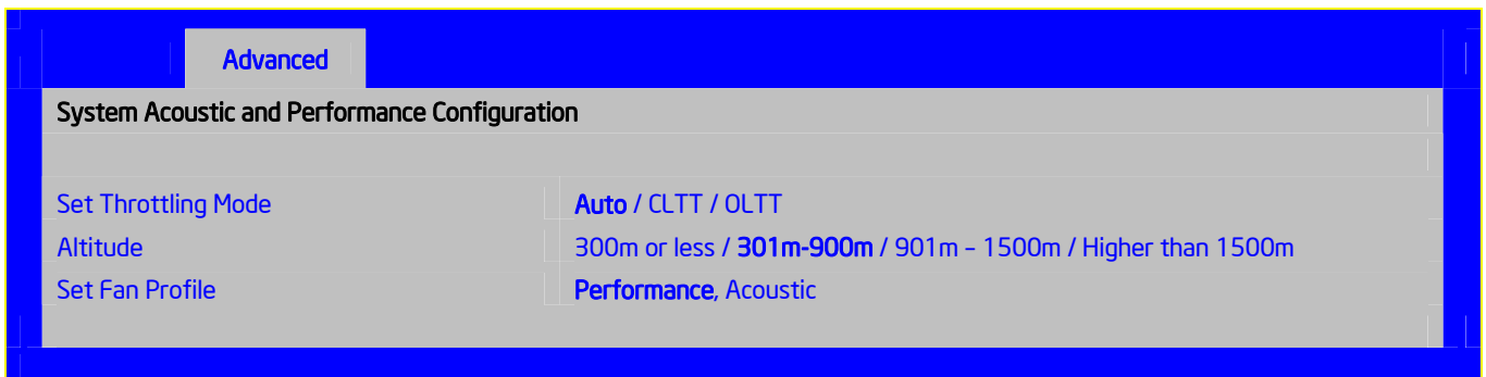
Figure 31. Setup Utility — System Acoustic and Performance Configuration Screen Display
