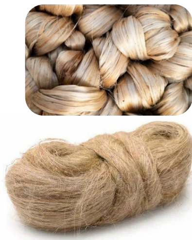
Figure 3. Flax and jute fibers (properties are depending on aspects, for example: harvest time, region, etc.), [13], [14]
