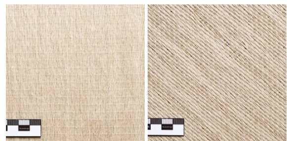
Figure 7. Bcomp products for composite manufacturers. Left side: unidirectional flax fabrics, right side: ± 45 bi-axial flax fabric [38]
