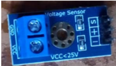
Figure 3. B25 Voltage sensor
