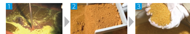
Procedures of the refinement ① Apply a special solution to extract gold by dissolution and reduction reaction. ② Filtrate and dry the extracted solution to turn it into powder (gold powder). ③ Melt the gold powder at a high temperature and put it in cold water to turn the gold into grains.
