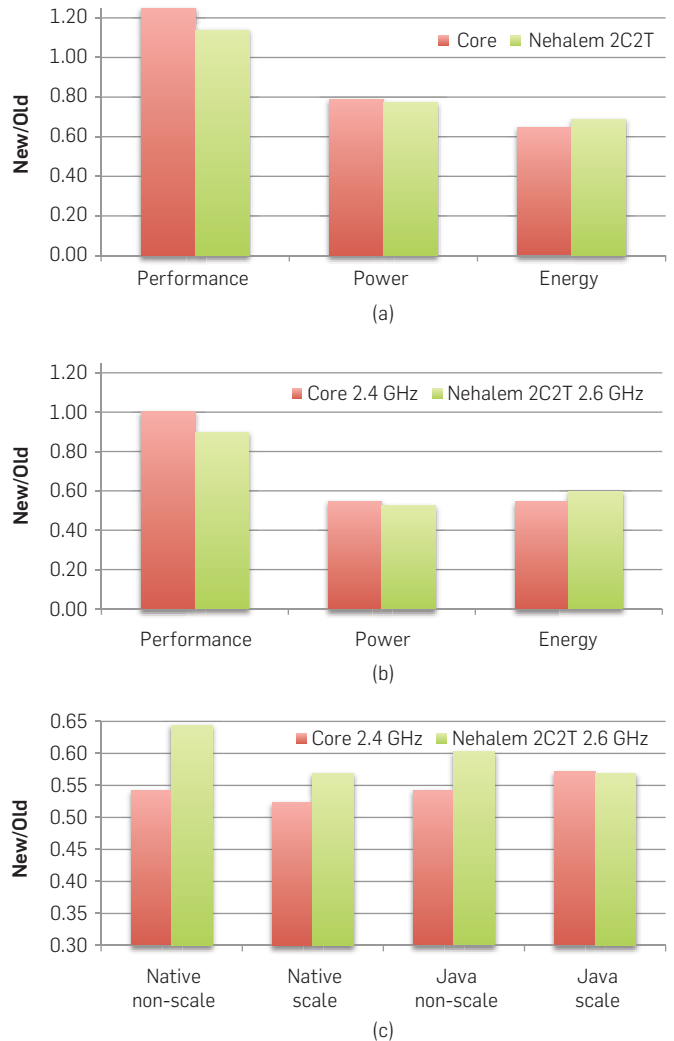
Figure 10. Die shrink: microarchitectures compared across technology nodes. “Core” shows Core 2D (65)/Core 2D (45) while “Nehalem” shows i7 (45)/i5 (32) when two cores are enabled. (a) Each processor uses its native clock speed. (b) Clock speeds are matched in each comparison. (c) Energy impact with matched clocks, as a function of workload. Both die shrinks deliver substantial energy reductions.
