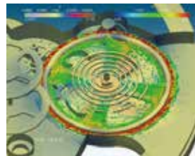
Evaluating the impact for the time accuracy with airflow simulations of the interior of a mechanical watch
