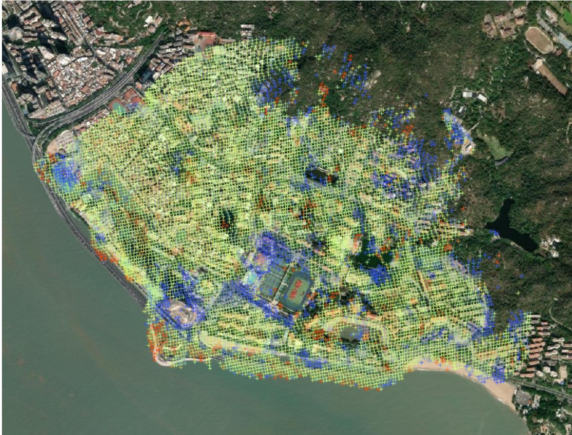
Figure 6 SBAS derived displacement velocity in vector format
