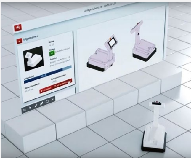
Factory Overview software panel for monitoring and controlling UNITR
