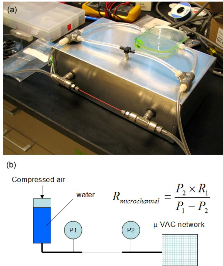
**Supporting Information Figure 1** (a) Image of the high-pressure flow meter apparatus used in this study. (b) Schematic illustration of this high-pressure flow meter.
