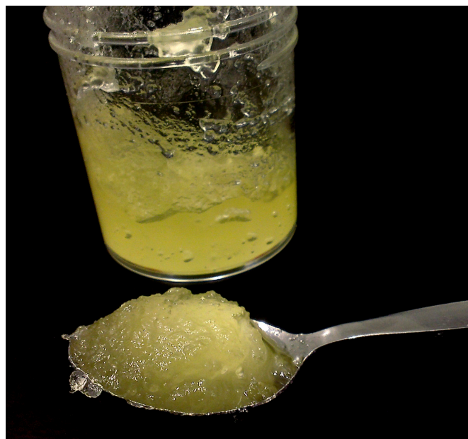
Fig. S1. Photograph of an organogel with 98 %wt liquid oil prepared by shearing oil-sorbed cryogels.
