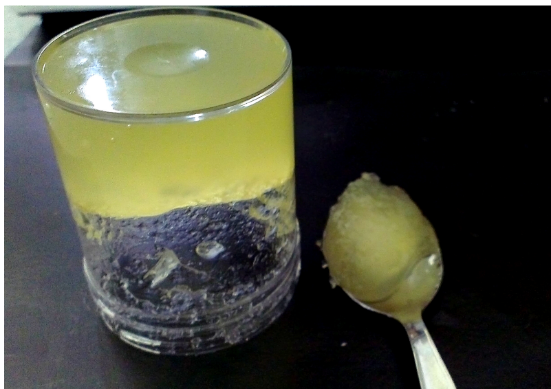
Fig. S5. Photograph of an organogel with 98 %wt liquid oil stored at 5°C for over 3 months. No oiling out or polymer sedimentation was observed on storage.
