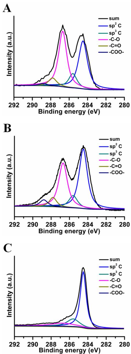
**Fig. S5** Fig. S5. Curve fit of C1s spectra of (A) GO, (B) RGO<sub>7/3</sub>, and (C) RGO<sub>9/1</sub>.
