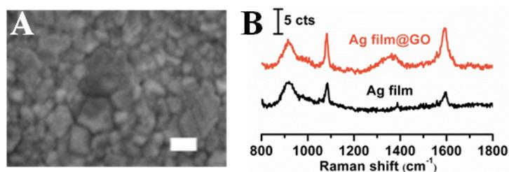
**Fig. S3.** (A) SEM images of Ag film. The scale bar is 100 nm. (B) The corresponding SERS spectra of 4-MBT adsorbed on Ag film (black line) and Ag film@GO (orange line).
