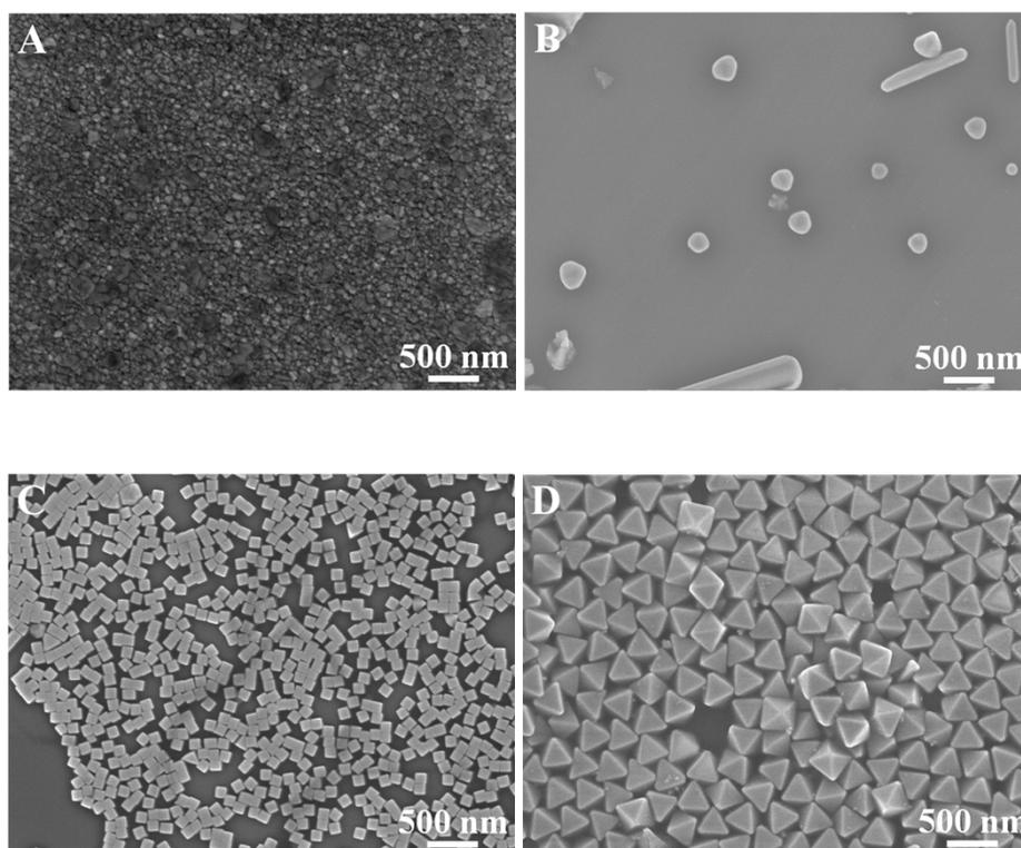
**Fig. S2.** SEM images of (A) Ag film fabricated by vacuum thermal evaporation, (B) Ag nanospheres, (C) Ag nanocubes, and (D) Ag octahedra.
