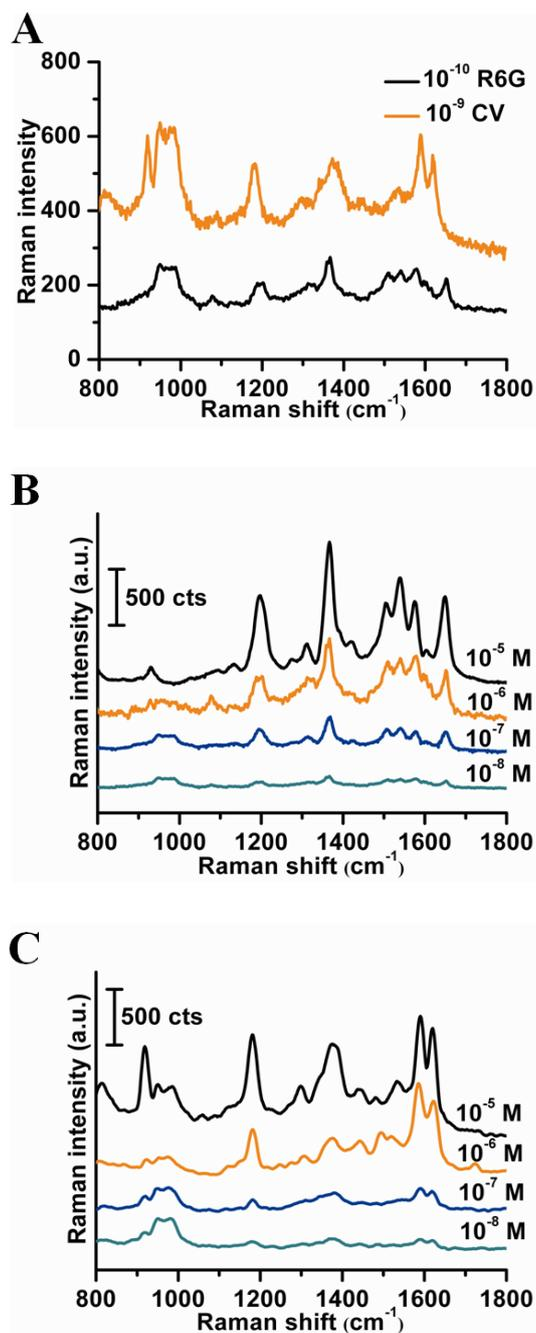
**Fig. S6.** (A) SERS spectra of  $10^{-10}$  M R6G and  $10^{-9}$  M CV deposited on Ag octahedron@GO. SERS spectra of R6G (B) and CV (C) on deposited Ag octahedron by soaking in the solution with different concentrations. For both R6G and CV, the concentrations from top to bottom are  $10^{-5}$ ,  $10^{-6}$ ,  $10^{-7}$  and  $10^{-8}$  M.
