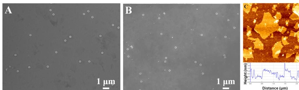
**Fig. S4.** SEM images of (A) GO@Ag octahedra and (B) Ag octahedra@GO hybrid on Si substrates. (C) AFM image and corresponding height profile of GO@Ag octahedra. The areas of Ag octahedra are carefully avoided due to the great disparity in the cross-sectional profiles of Ag octahedra and GO.
