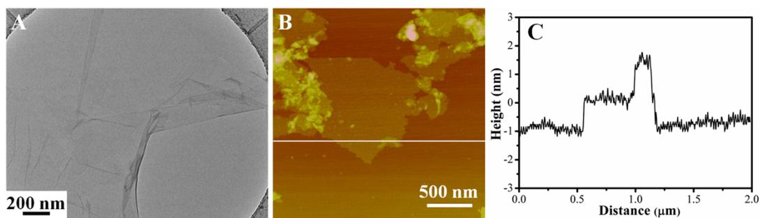
**Fig. S1.** (A) TEM image of GO, (B) AFM images and (C) corresponding height profiles of GO on silicon substrates.
