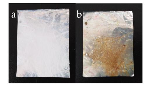
**Fig. S3.** Optical photograph of PC/Ag hybrid substrate: (a) before reduction; (b) 410 s chemical reduction.
