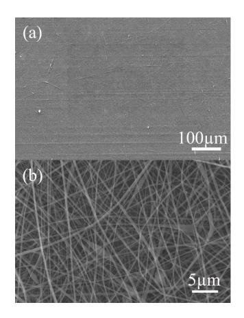
Fig. S1. SEM images of pure PC nanofiber membrane (14 wt% PC): (a)500×magnification;(b)10000×magnification.
