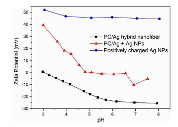
**Fig. S5.** Zeta potential of positively charged Ag NPs, PC/Ag hybrid nanofiber and PC/Ag+Ag substrate.
