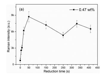
**Fig. S2.** Peak Intensity of 10<sup>-6</sup> M 4-ATP recorded on hybrid substrate with different chemical reduction time (0.47 wt% AgNO<sub>3</sub> content).
