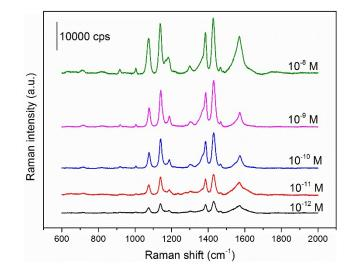
**Fig. S6.** SERS spectra of different concentrations of TNT collected on the PC/Ag+Ag substrate.
