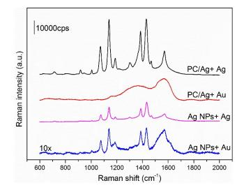
**Fig. S7.** Raman spectrum of 10<sup>-6</sup> M TNT on different substrates.
