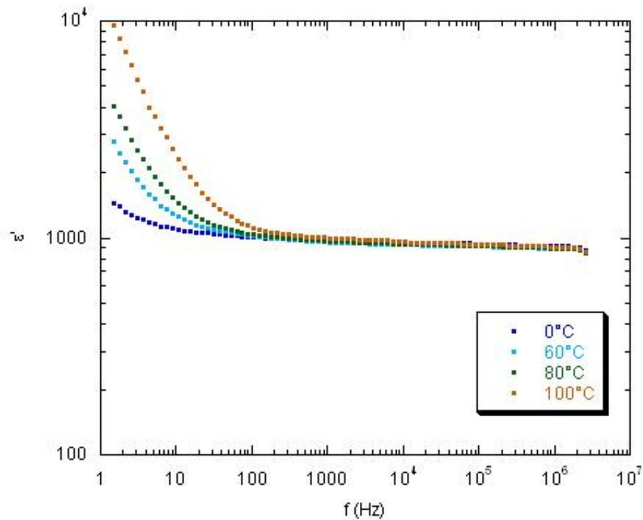
Figure S7. Real part of the permittivity for HEOx-2%Li with Li-electrodes
