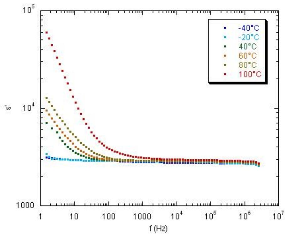
Figure S6. Real part of the permittivity for 2%Li HEOx as a function of frequency, for various temperatures.
