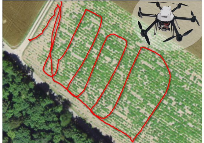
Fig. 1: The top view of the environment where the experiments presented in this paper were carried out. The red line represents the trajectory of one of the performed flights. The platform used is the AscTec Neo hexacopter, shown in the inset.
