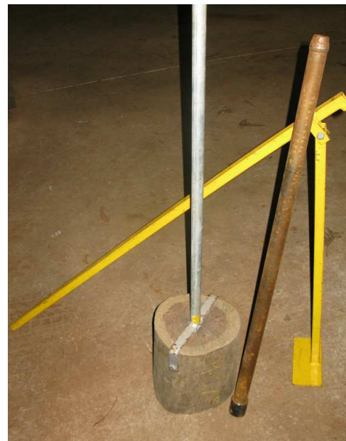
Figure 3. Soil hand coring kit comprising thin walled coring tube (1 m length), extraction jack and wooden hammer.
