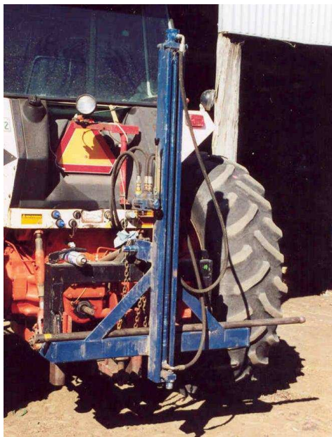
Figure 2. Soil coring rig attached to a tractor and utilising its hydraulic system to push thin walled coring tubes to a depth of 1.5 to 1.8 m.
