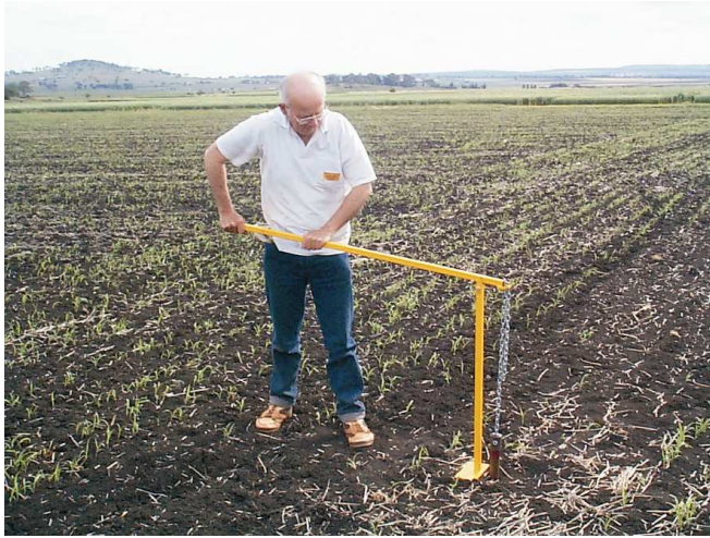
Figure 4. Extracting a core from a depth of 1 m using the extraction jack.
