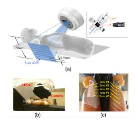
The CELSI technique employed by the researchers uses sheet-shaped radiation beams from a LINAC to produce Cherenkov photons. These photons excite probe luminescence in a volume confined primarily to the irradiation sheets. By shaping the x-ray beam into a thin sheet, images of Cherenkov-excited luminescence from a planar slice within the tissue can be acquired. A series of luminescence images is taken at different depths, thus providing a three-dimensional volumetric rendering.<sup>20</sup>
