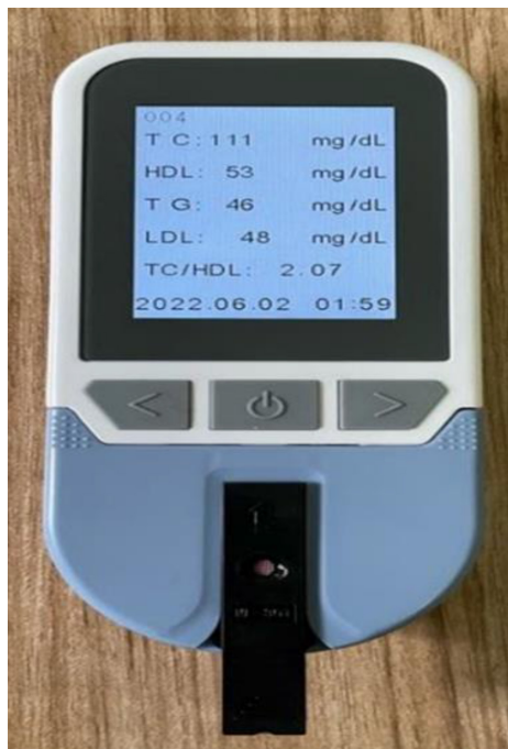
Figure 1. Cholchek™ is a device for measuring systemic Total Cholesterol, HDL, LDL & Triglyceride levels in the body (image from actual device taken through author's mobile phone)
