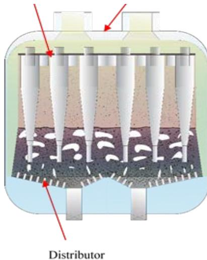
**FIGURE 6:** A SCHEMATIC OF THE PFB HX DRIVING THE ABCC POWER CYCLE.
