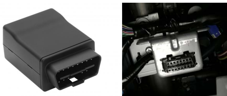
Figure 1. Telematics device (left, photo from CalAmp 2017) and Subaru Forester OBD-II port (right, photo by Cabell Hodge, NREL)
