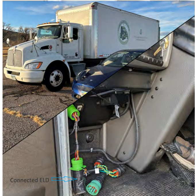
Fig. 4: Research Truck (top) with ELD plugged into Diagnostic Port and hanging to the right of the door edge (bottom).
