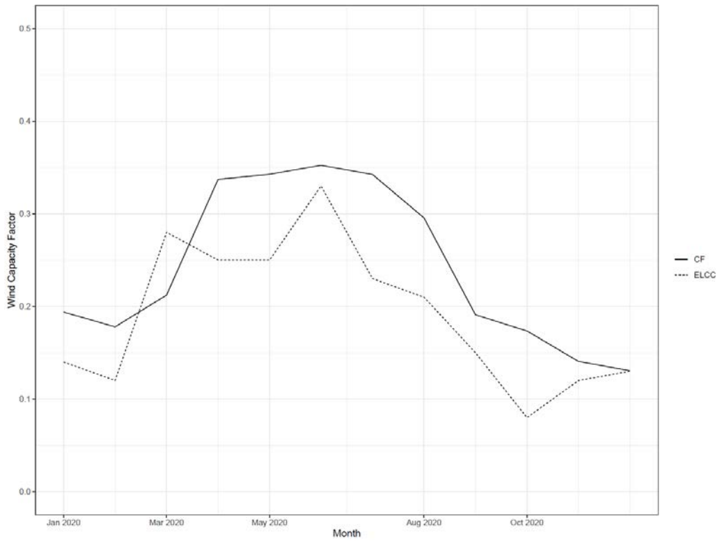
Figure 6(a): Monthly Average Wind Capacity Factor and ELCC Value for Firm Capacity for 2020
