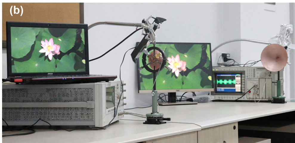
Figure 10. (a) The experiment setup of the dual OAM communication link. The l=+3 channel carries the square wave modulated millimeter-wave signal, and the l=-3 channel carries the HD video signal. (b) The experimental photo to demonstrate the successful transmission of two independent channels. The picture on the screen is extracted from the video, Copyright The Admission Office of Zhejiang University.
