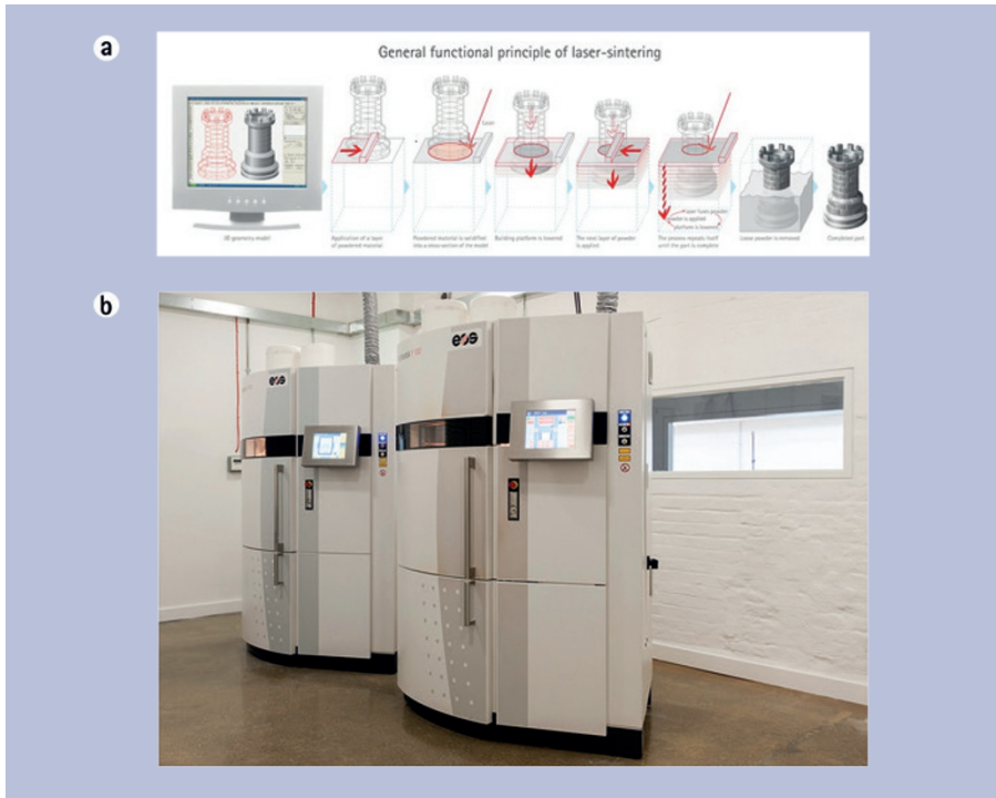
Fig. 10 (a) diagram of SLS printing process (diagram courtesy of EOS, GmbH). 61 (b) Industrial SLS apparatus (image courtesy of www.digits2widgets.com)
