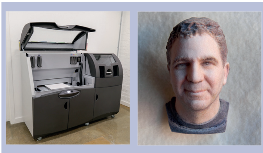
Fig. 11 Industrial powder binder printer and example bust of author captured with 3D photography and printed in full colour plaster of Paris (courtesy of www.digits2widgets.com)
