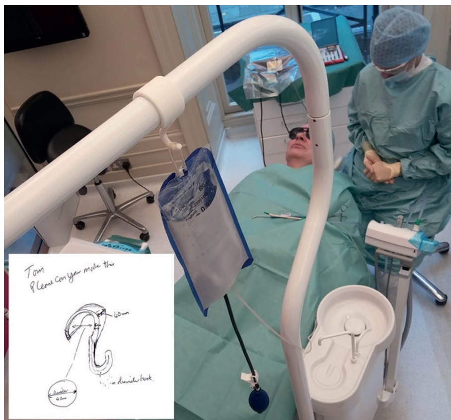
Fig. 9 Back-of-envelope design, leads rapidly to a functional prototype for a 3D printed saline bag holder, fitted to dental chair
