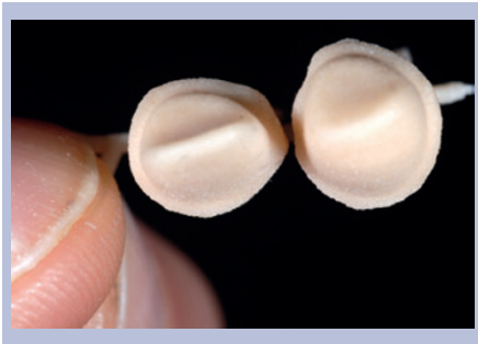
Fig. 7 SLS printed prepared teeth, printed from data from an intra oral scanner
