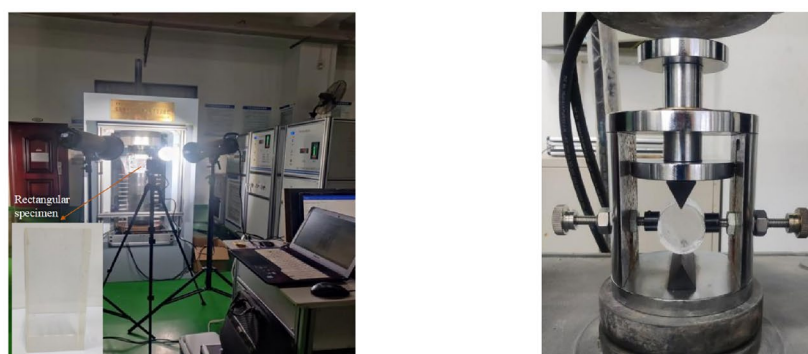
(a) Compression testing machine and rectangular specimen (b) Brazilian splitting test fixture and specimen
