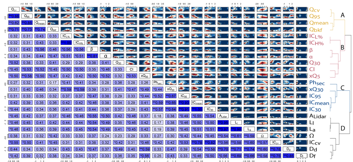
Figure 7. Atmospheric (CI), landscape (IC, Ph_{sec} ), river ( \alpha, \beta ) and flow (Q, xQ) properties are correlated to different degrees (values of correlation -dCor - close to 0 represent no correlation, and 1 represent perfect correlation) [Lower triangular matrix in the image; shades of blue highlights the correlation strength, from weak (light) to strong (dark)], with some strong non-linear dependence emerging between specific variables [ dCor values marked with ** are statistically significant at the 0.05 level, values marked with * are significant at the 0.1 level, values marked with ° are significant at the 0.2 level.] The interaction between variables [open circles in the upper triangular matrix] reinforces or offsets the decadal trends of exceedance of extreme flows [upper triangular matrix; shades of red represent progressively increasing decadal trend, white represent no trend, and shades of blue represent decreasing trends]. We used a kernel density estimation (KDE 138 ) to display in a non-parametric way the decadal trend for each 2 way combination of landscape indicators, using the start positions of each variable within the scatterplot. The correlation strength allows to define cluster of variables (dendrogram) that are more closely related. Elements that are merged at a lower height (shorter branches in Fig. 7) are more similar (dependent) than Elements that merge at greater height. It is possible to identify four separate clusters, including flow properties (A), reach properties, climate and flood hazard (B), morphodynamics properties (C), and scale-dependent parameters (D). Figure was arranged using customized scripts on Rstudio Version 1.2.1335. See Data and software availability for details.
