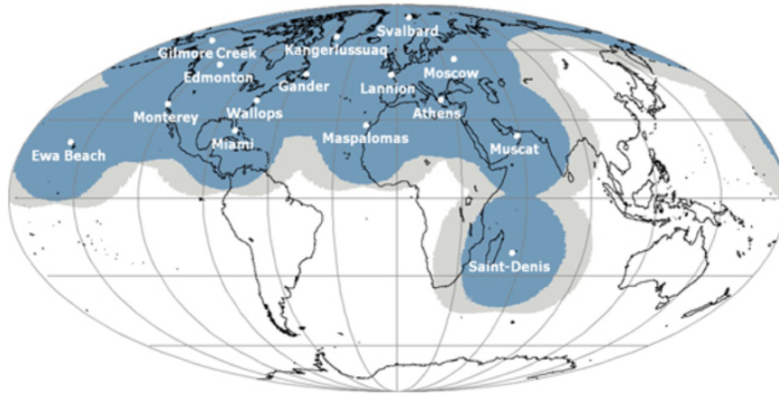
Fig. 8. Map of EUMETSAT Advanced Retransmission System (EARS) stations that receive AMSU/MHS data directly from the over-passing NOAA and MetOp satellites, and retransmit the data to EUMETSAT Headquarters. The color coding indicates the percentage of the actual satellite passes over a given geographical region – i.e., swaths that can be received by the proposed station network. Light grey corresponds to 0–50 % and blue corresponds to 50–100 % (here, 100 % indicates that every time the region is in the field of view of the instrument, then the image data will be received by the network, while 50 % indicates that, on average, every second pass covering the region will be received). (Courtesy of EUMETSAT: http://www.eumetsat.int/website/home/Satellites/CurrentSatellites/Metop/RegionalDataService/EARSATOVs/index.html .)
