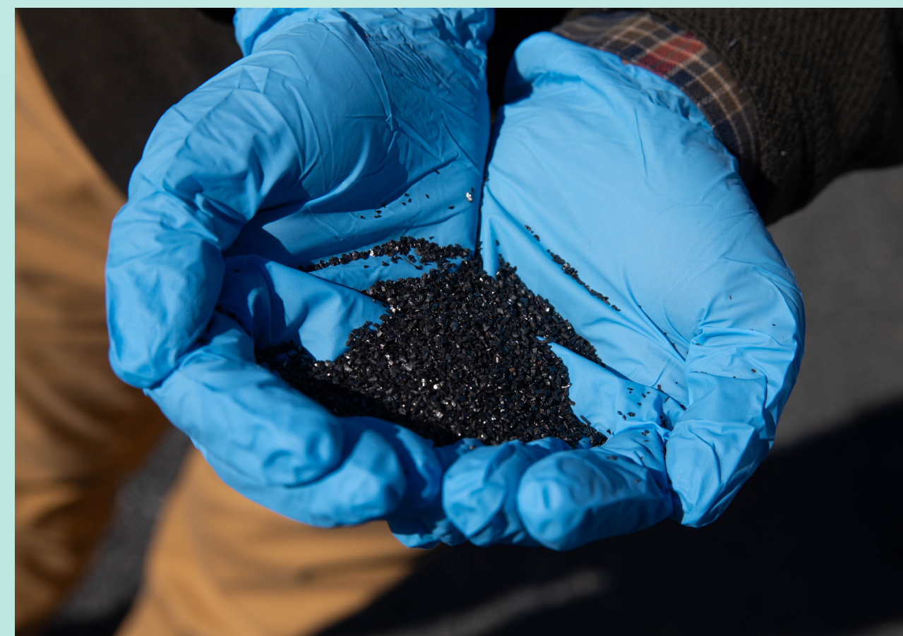
Adsorbent materials often contain activated carbon that captures PFAS from surface water.
