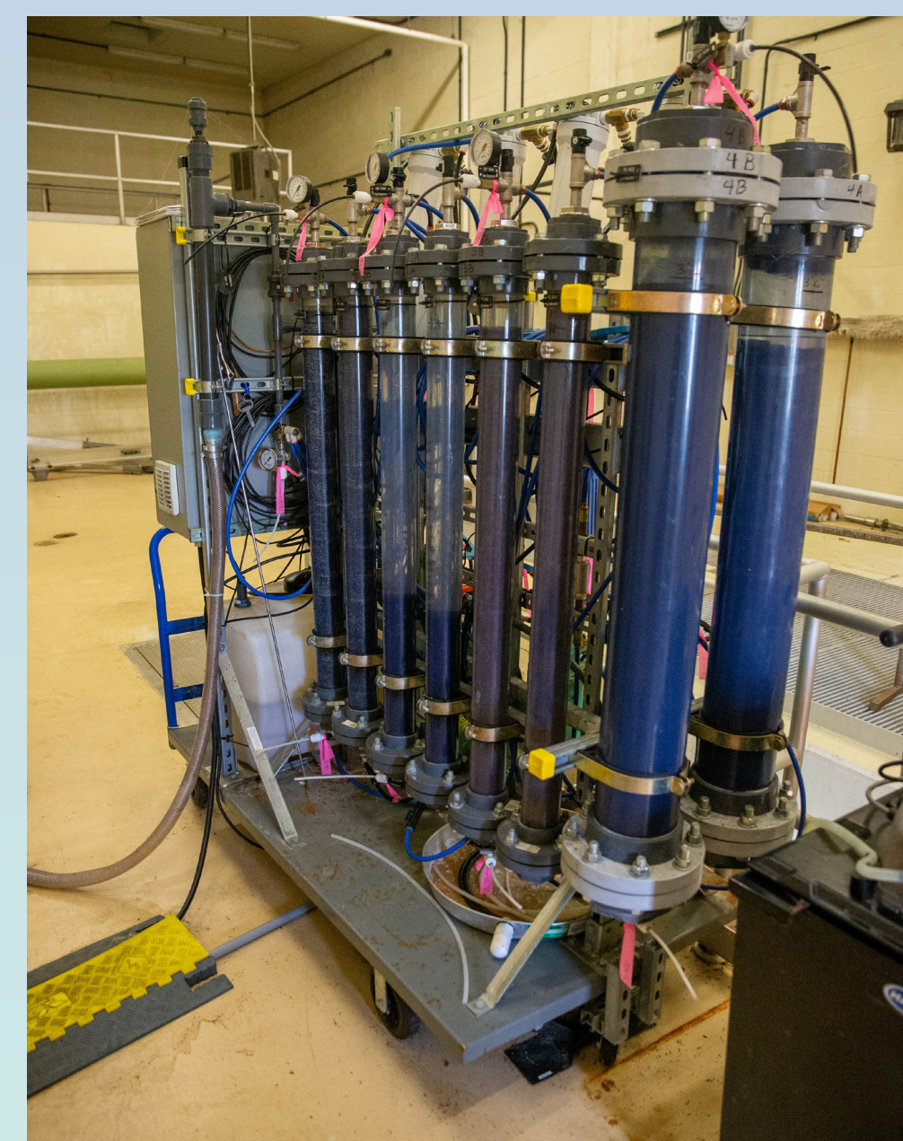
NASA testing apparatus that is being used to evaluate effectiveness of various adsorbents to remove PFAS from the Wallops WWTP effluent.
