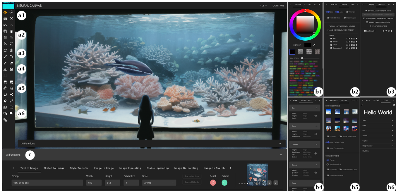
Figure 4: The user interface of Neural Canvas. a1) Mode selection buttons. a2) General operation buttons. a3) Canvas operation buttons. a4) Brush operation buttons. a5) Image operation buttons. a6) Projection operation buttons. b1) The brush parameter panel. b2) The layer manager panel. b3) The camera manager panel. b4) The 3D primitive manager panel. b5) The environment control panel. b6) The text box panel. c) AI function panel: this drop-down panel consists of multiple tabs of different AI functions.
