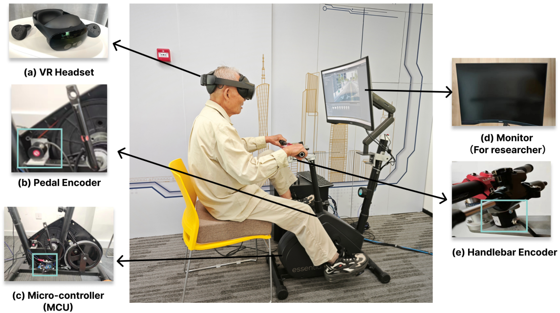
Fig. 1. SilverCycling System Components and the main working process. The setup includes a Modified Indoor Cycling Machine equipped with a (e) Handlebar Encoder and a (b) Pedal Encoder to detect physical movements. (c) MCU reads input signals and subsequently transmits these signals to the PC. (a) The users wear the VR headset and movement is synchronously mapped to the camera movement within the VR environment in the headset. (d) The monitor is used for observation by researchers.
