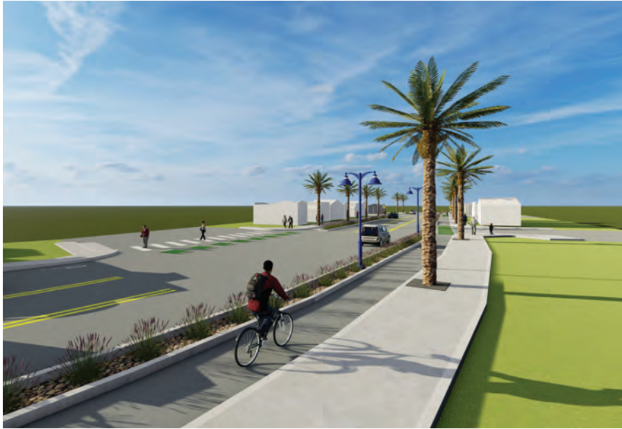
Proposed Class IV separated bikeway with transition striping, pedestrian lighting, and high-visibility crosswalks; looking east
