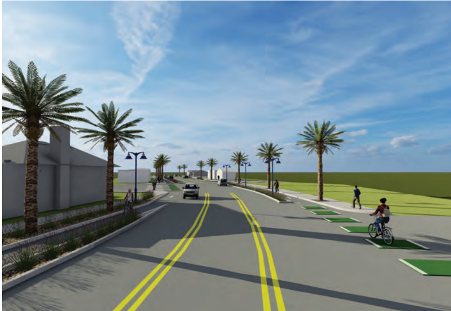
Proposed Class IV separated bikeway with transition striping and pedestrian lighting, looking west
