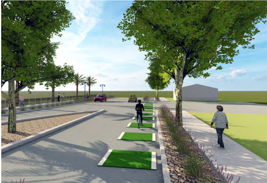
Proposed Class IV separated bikeway with transition striping placed at intersections or busy driveways; looking east
