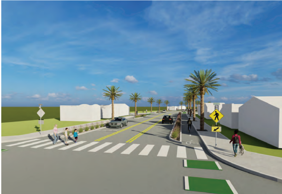
New north-south crossing with rapid rectangular flashing beacons, high-visibility crosswalk, and signage; looking east
