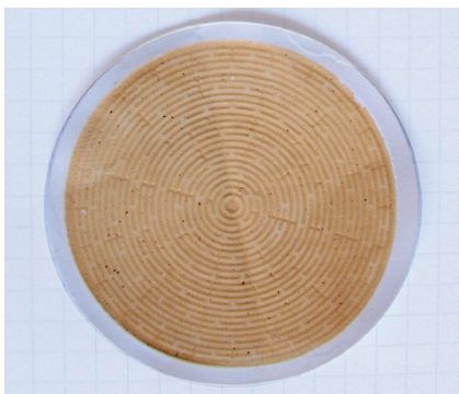
SDI Filter before UF System
