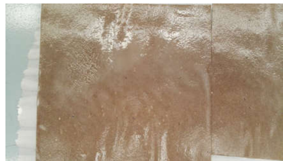
Figure 2: Sprayed MFC on the packaging paper
