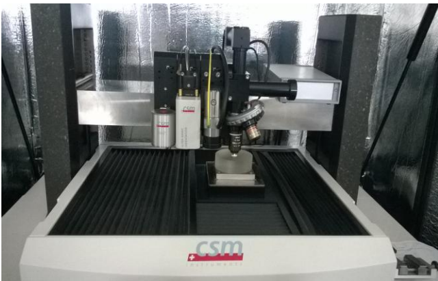
Figure 2: The snap shot of Micro Hardness Tester CSM Instruments UNHT loaded with \text{Na}_{0.5}\text{K}_{0.5}\text{NbO}_3 ceramic pellet
