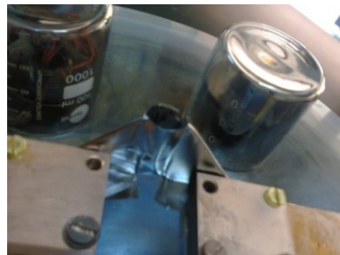
Figure 2: Tantalum boat connected between copper electrodes
