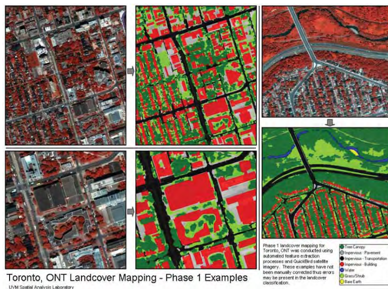
Figure 7. Classification of satellite imagery to produce a digital land cover map (Credit: University of Vermont Spatial Analysis Laboratory).
