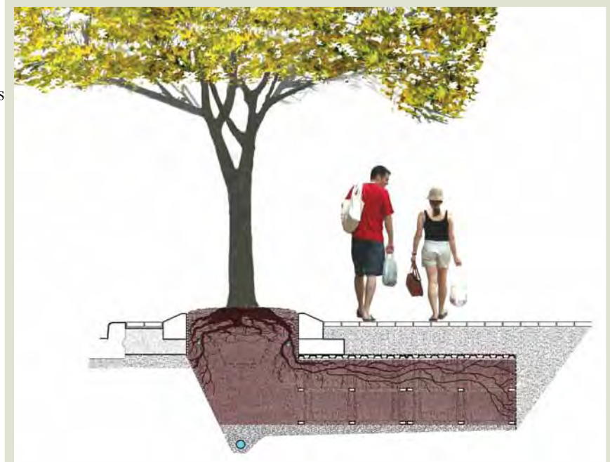
Figure 35. Silvacells being used to increase soil volumes for tree planting in a commercial area (Credit: Urban Forestry).
