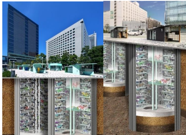
Figure 3. Automated underground bicycle parking at Kyoto and Shinagawa stations
