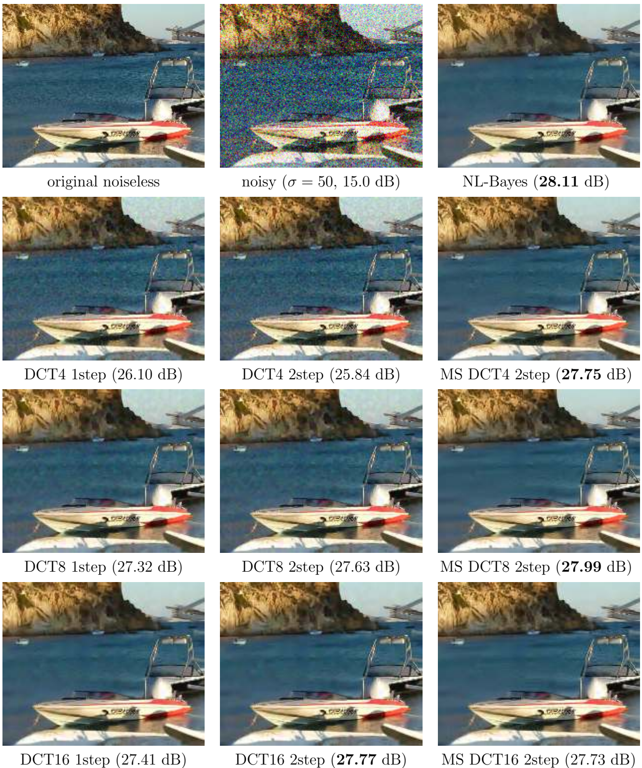
Figure 7: Results and PSNR of DCT denoising without oracle (1step), with oracle (2step), and with multiscale (algorithms 2, 1, 5), using patches of sizes 4 \times 4 , 8 \times 8 , and 16 \times 16 . For each patch size the optimal parameters from Table 1 were used.
