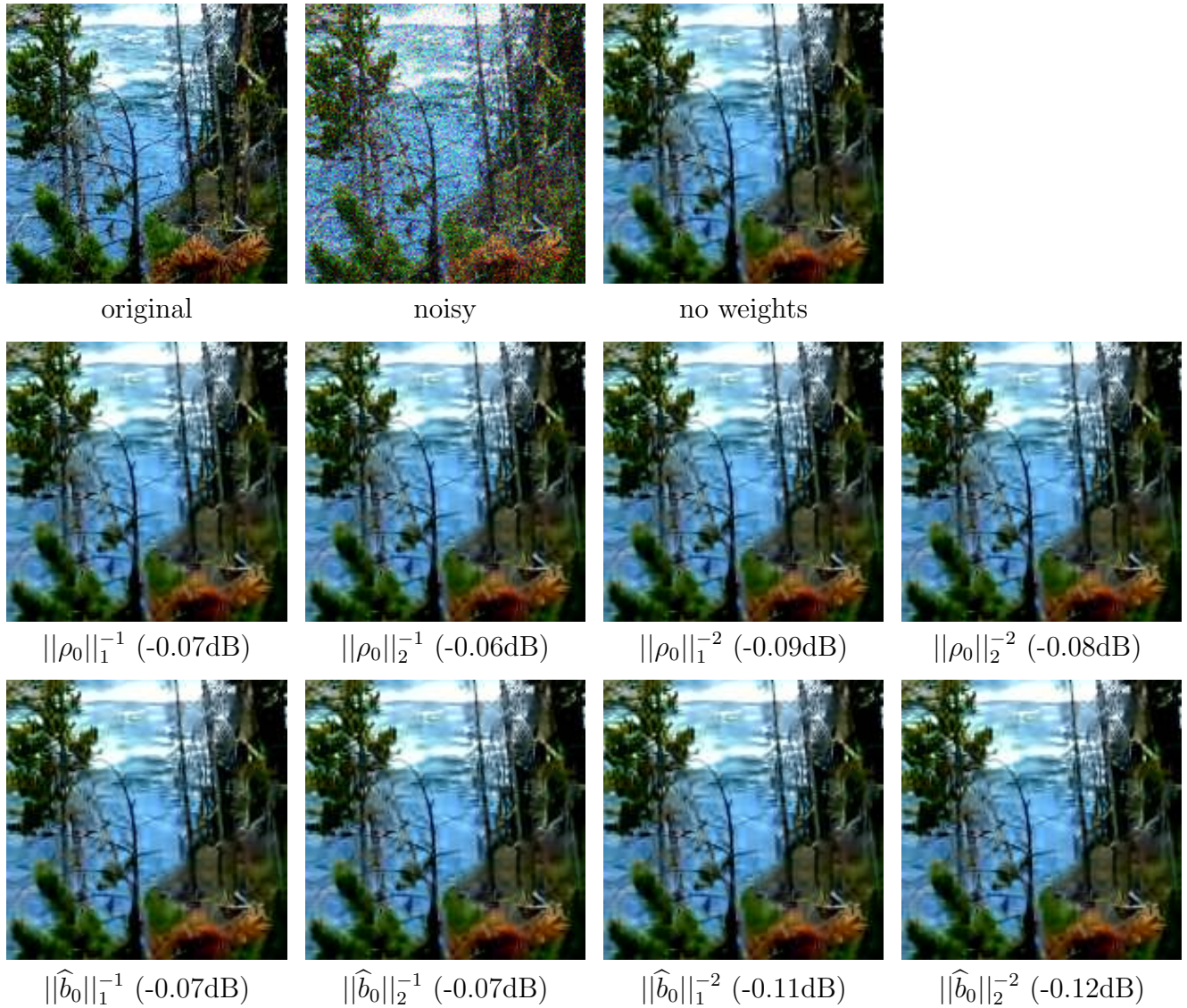
Figure 11: Effect of different aggregation weights on the MS DCT algorithm (with 8 \times 8 patches) with noise \sigma = 50 . This image illustrates a case in which aggregation weighting results in PSNR loss, usually in images dominated by textures. The PSNR increments are computed with respect to the output of the algorithm without aggregation weights. For this image all the aggregation weights produce similar results, which are also barely distinguishable from the non-weighted version. The contrast on these crops has been increased to highlight the artifacts (better seen in the electronic version).
