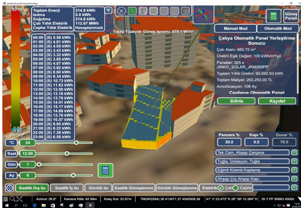
Figure 12. Solar estimation for the selected building rooftop.
