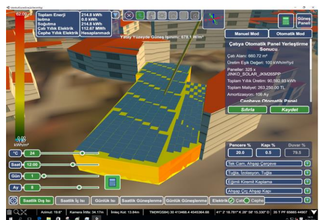
Figure 11. Potential solar panel for a building rooftop.
