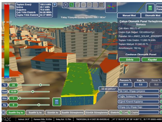
Figure 13. Solar estimation for the selected building rooftop and façade (potential solar panel).
